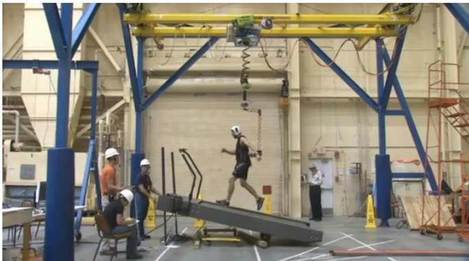
ARGOS (Active Response Gravity Offload System)
