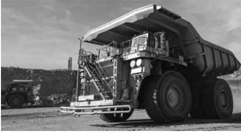
Mining trucks are monstrous machines that guzzle fuel at a scarcely believable rate. Weighing 220 tonnes, they can get through 134 litres of diesel every hour. Little wonder then that mining companies are focusing their attention on these vehicles as the first step to reducing their carbon footprint.
